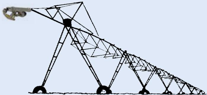
**APPLICATION:** Install at the end of center pivot systems for automatic flushing at start-up and shut-down — or, configure with an electric solenoid interfaced with the center pivot for automatic flushing while system is operating.
